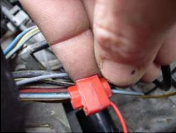
(NOTE - The displacement connector is supplied purely as a convenient solution. If you have a preferred method for splicing these wires then feel free to do so. Splicing into the wire directly via a butt connector or via soldering can produce a better union. Be sure to insulate all connections properly.)
