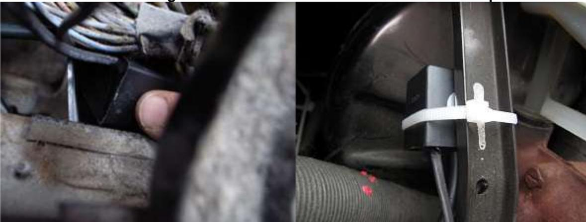
3. Locate the grey wire on the back of the headlight switch.
