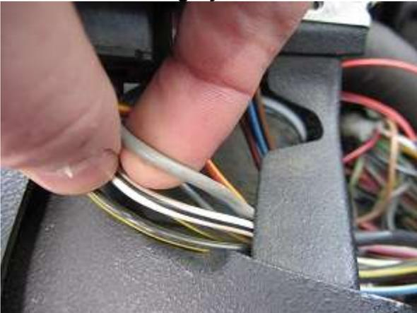
(Note – tapping into the gray wire will keep the backlighted portion of the gauges illuminated any time the headlight switch is in the “on” position regardless of the ignition key position.)
