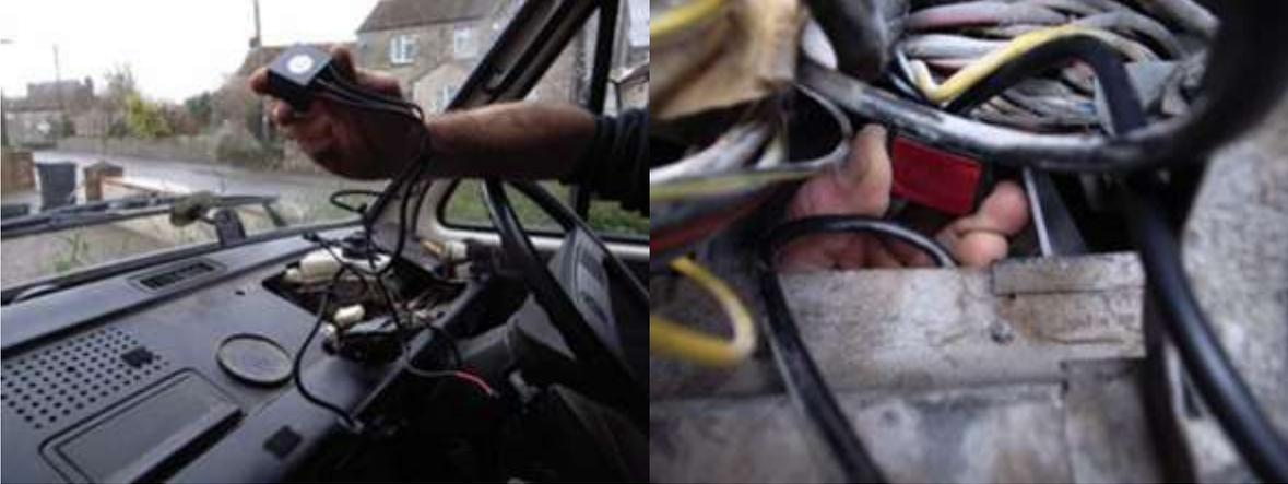
2. Place the ballast somewhere it won't rattle around. The space behind the wire loom, just inside the steering column shroud works well. You could also zip tie it to the dash board brace.
